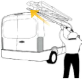
2 With both hands, insert the handle into the Max Rack and turn to secure.
