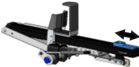
Slide plastic pad along the rail to be under ladder frame.
