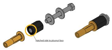
**b.** Insert into drilled hole.
