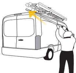
**3** With both hands, insert the handle into the Max Rack and turn to secure.
