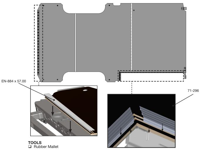
NOTE: Line up sill extrusion correctly before pressing it in. Use rubber mallet when needed.
