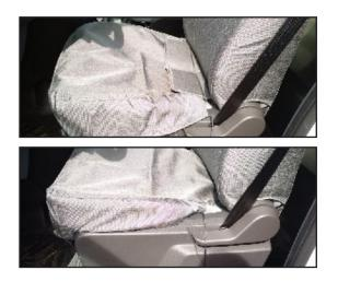
2.2.3 Push flap on top of cover between seat back and seat bottom.
