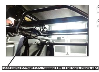
**2.2.8** Pull bottom flaps from front of seat bottom and attach to top flap.
