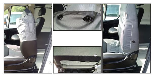
**2.1.1** Install Seat Back Cover. Ensure the tag inside the cover corresponds with the seat you are working on. Each cover will have a Driver or Passenger tag.
