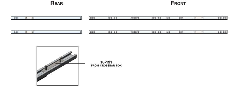
**2.1.2** Install the mounting tracks onto the roof of the van.
