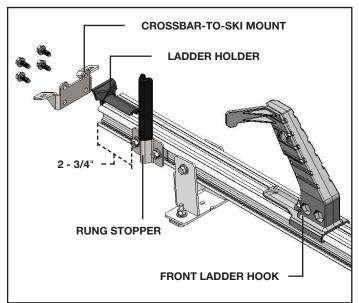
NOTE: Attach the front ladder hook, rung stopper and ladder holder to the crossbar before attaching the crossbar-to-ski mount.
