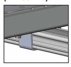
NOTE: Move the ladder hood in place, then tighten the bolts in the bracket.
