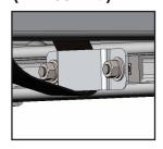
NOTE: Move the belt retainer to the center of the rung, then tighten the bolts
